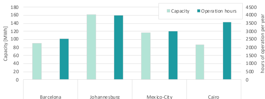
Figure 7: Comparison of annual capacity and operation hours for the four locations.
