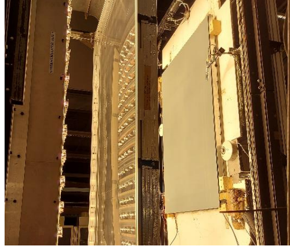
Fig 4: Laboratory measurement of the PVT collector as a façade collector in the solar simulator according to DIN EN ISO 9806
