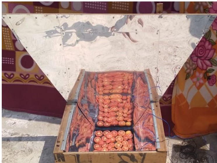
Fig.1b: Photograph of BISD with drying material (Sliced tomatoes)
