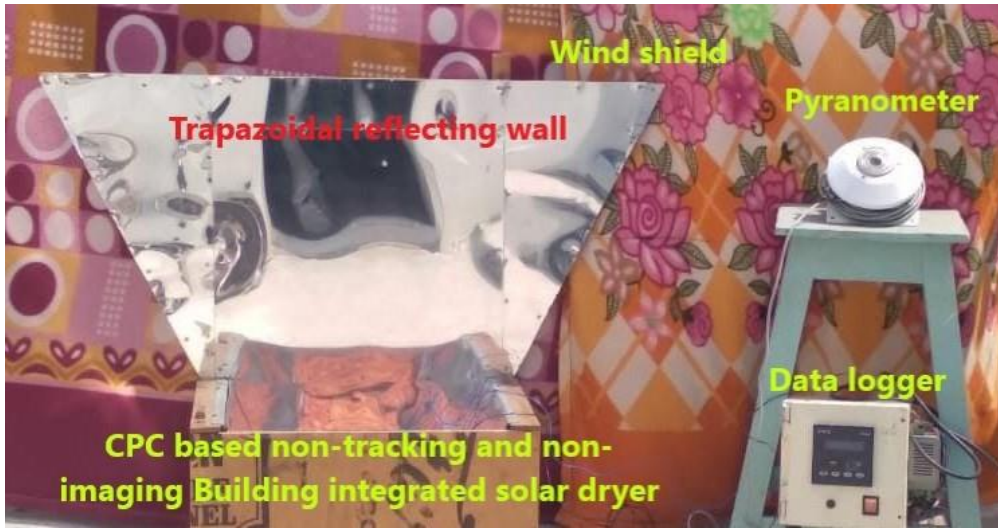
Fig. 1a: Photograph of test setup for BISD
