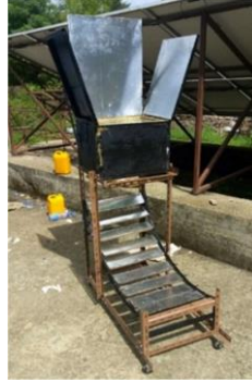
Fig. 3: photographic view of double exposure solar cooker
