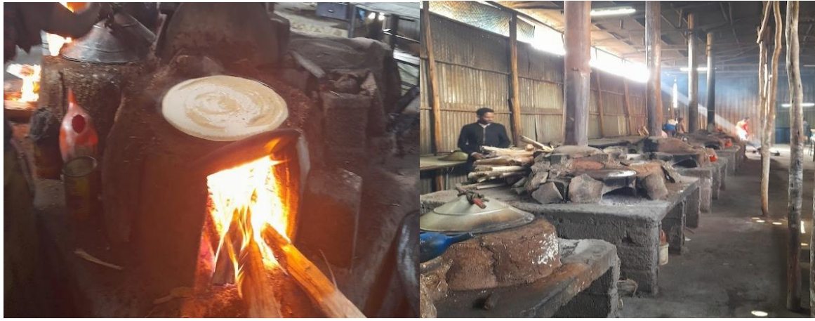
Fig.1: Injera baking system currently in use at Bahir Dar University
