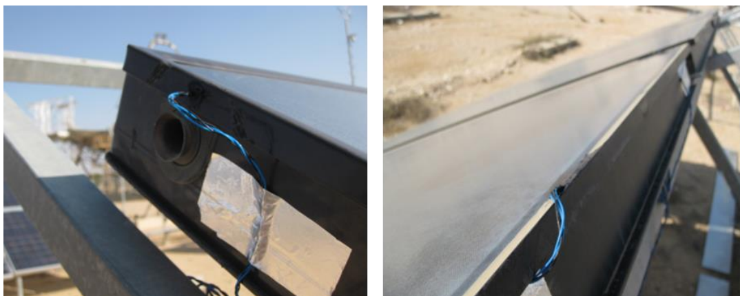
Figure 1 Thermal solar collectors prepared with thermocouple to measure the adhesive joint temperature position top left (left) and position top middle(right) alt maritime exposition
