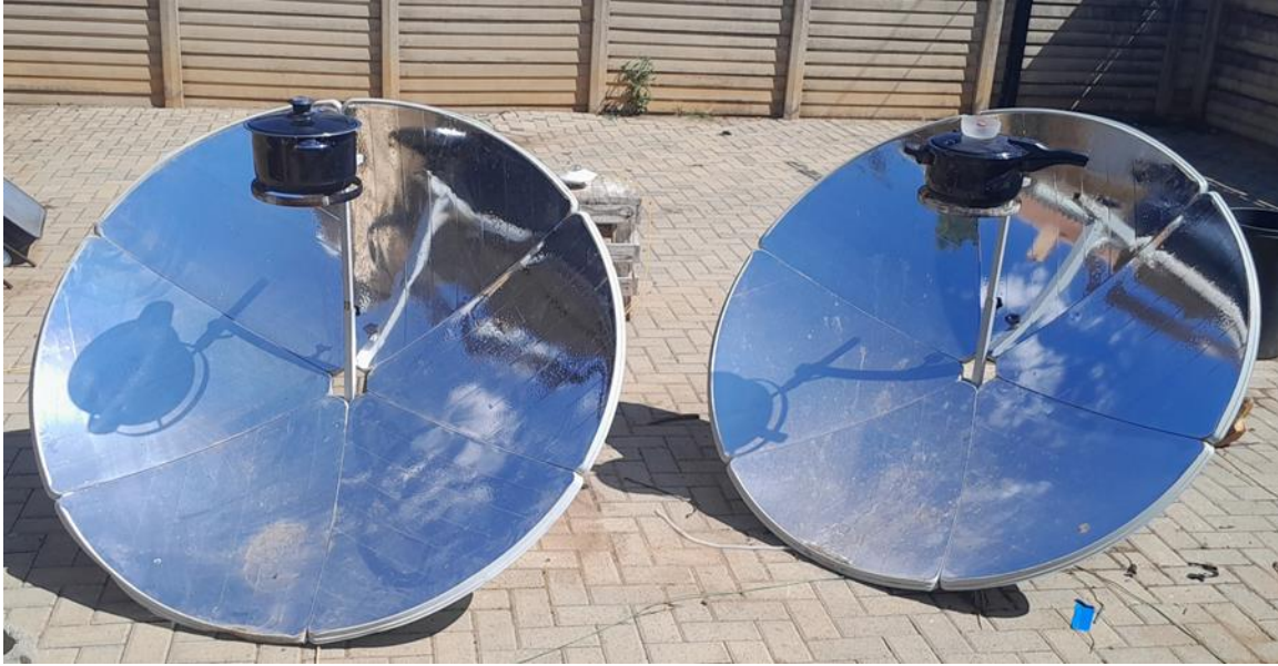
Fig. 2: A photograph of the 1.5 m parabolic dish solar cookers with the two specialised cooking pots just before experimental tests
