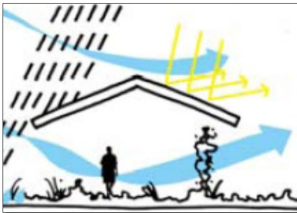
Figure 1: Strategies in tropical Climate: solar protection, daylight, ventilation, shades.
