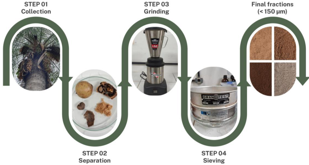
Figure 1: Preparation steps of macaúba fractions: collection, separation, grinding, and sieving (Author, 2025).
