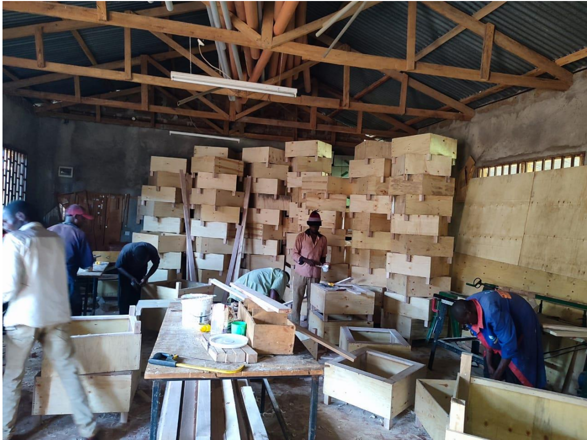
Figure 2: Picture from the production phase of Standard-size ULOG solar ovens manufactured at Kiini Institute, Chuka, Kenya for the 2025 annual implementation cycle of this initiative. Photo credit: Eco-Impact Hub CBO.
