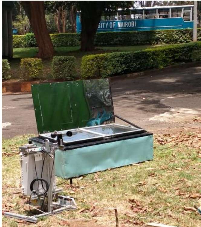
Figure 3: Picture of a Family-size ULOG solar box oven being tested using the SCI Performance Evaluation Process (PEP) solar cooker testing instrumentation at the Stove Testing Center, University of Nairobi, Nairobi, Kenya. Photo credit: Justus Muoki.
