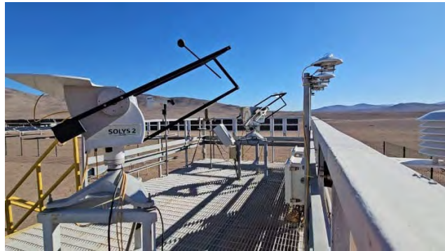
Figure 1: PSDA ground-based station, located in the Atacama Desert (24.09°S, 69.93°W) at 965 m a.s.l., with systems and radiometric instruments operating under extreme arid conditions.
