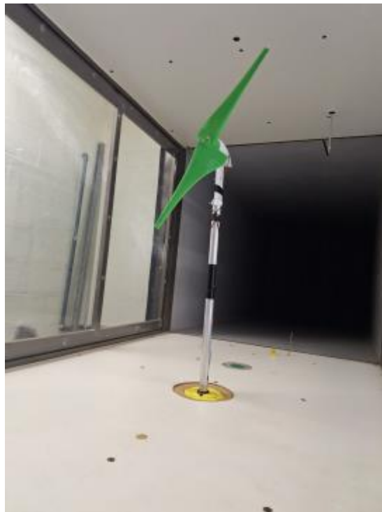
Fig. 2: 3D Printing in Wind Tunnel Test
