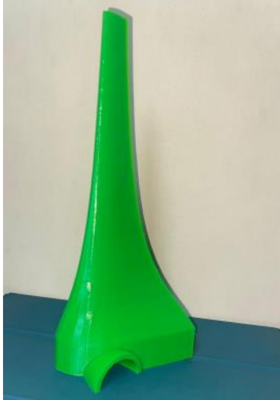
Fig. 1: 3D Printing of The GOE 770 Model
