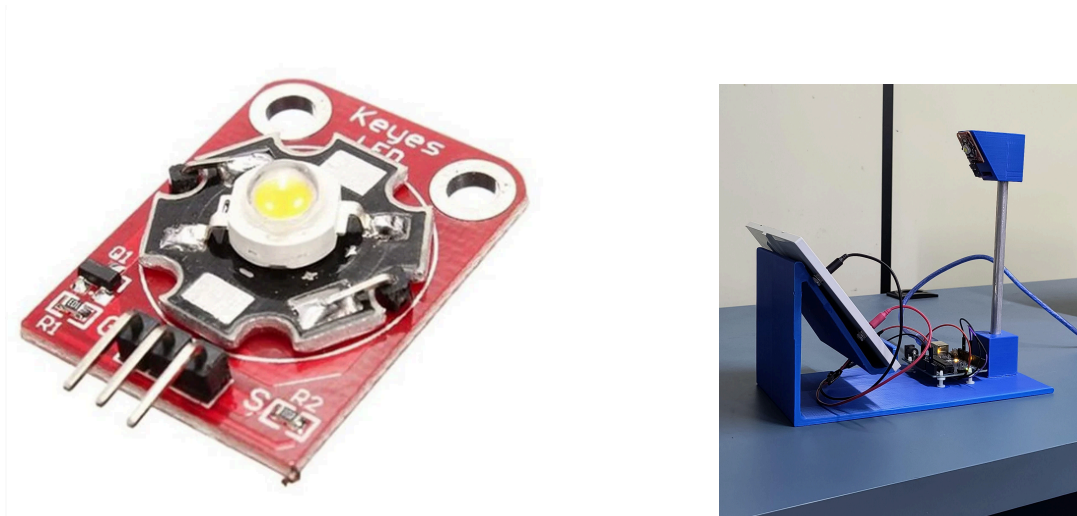
Fig.1: High-power LED module 3W used for PV panel excitation. (left); Physical mounting of the experimental setup. (right)
