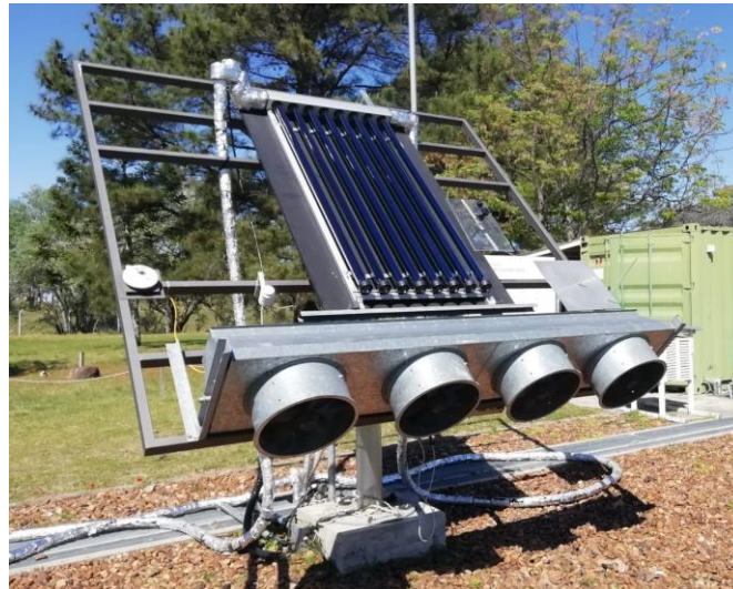
Figure 1: Assembly of the collector on the solar tracker of the test bench, figure extracted from Rodríguez-Muñoz et. al. 2024.
