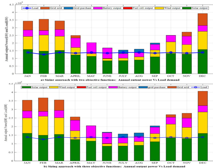
Fig. 5: Proposed NZEBs yearly output power status for both sizing techniques.
