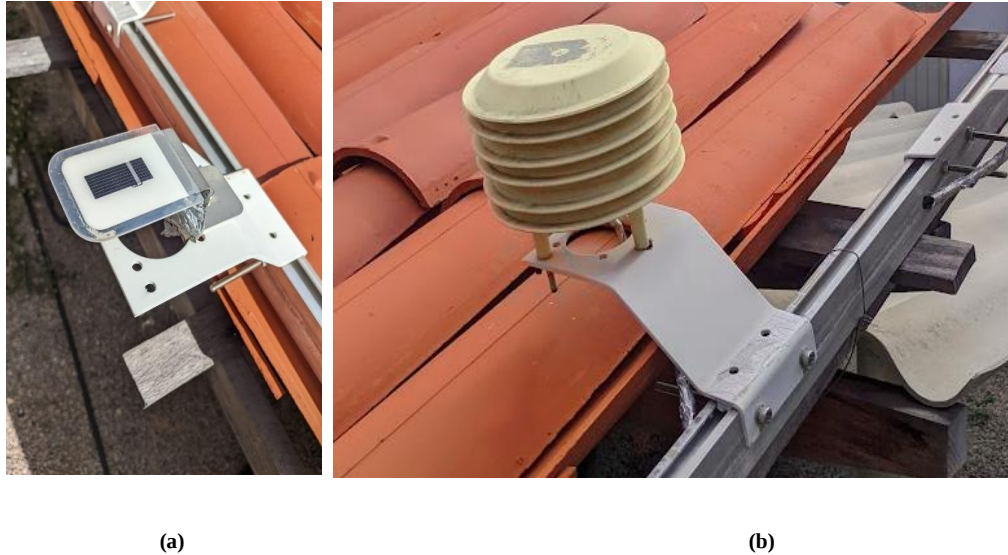
Figure 6: (a) SPEKTRON 210 sensor; (b) DHT22 sensor inside a weather shelter (Font: Author, 2025).
