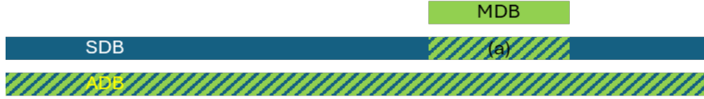
Figure 1: Site adaptation schematic: A one-year measured database (MDB) is used to find a function to adapt the overlap irradiance values (rectangle a) over a more extensive satellite database (SDB) of, e.g., 15 years. Then that function is applied to the entire SDB, and an adapted database (ADB) is obtained.
