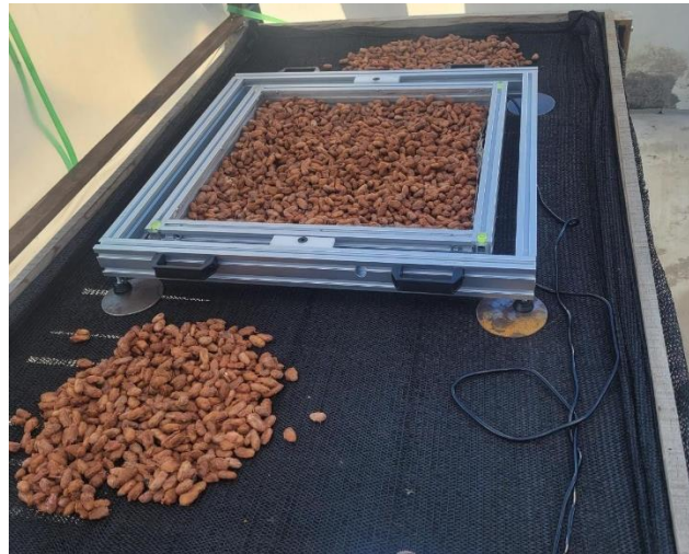
Fig. 3: Gravimetric humidity measurement system in the prototype greenhouse
