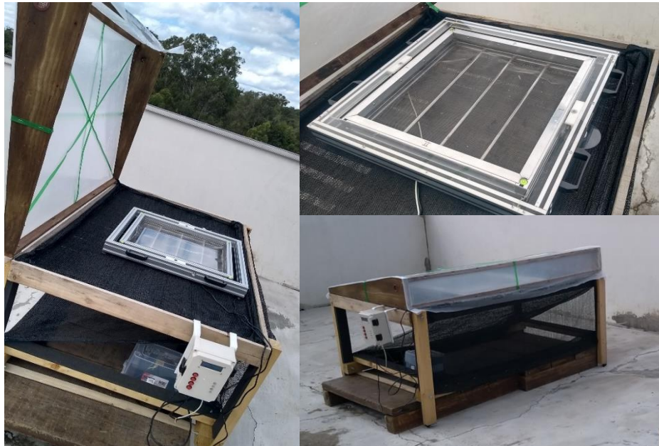
Fig.1: Greenhouse prototype with system to humidity measurement of agricultural products during dryer process.
