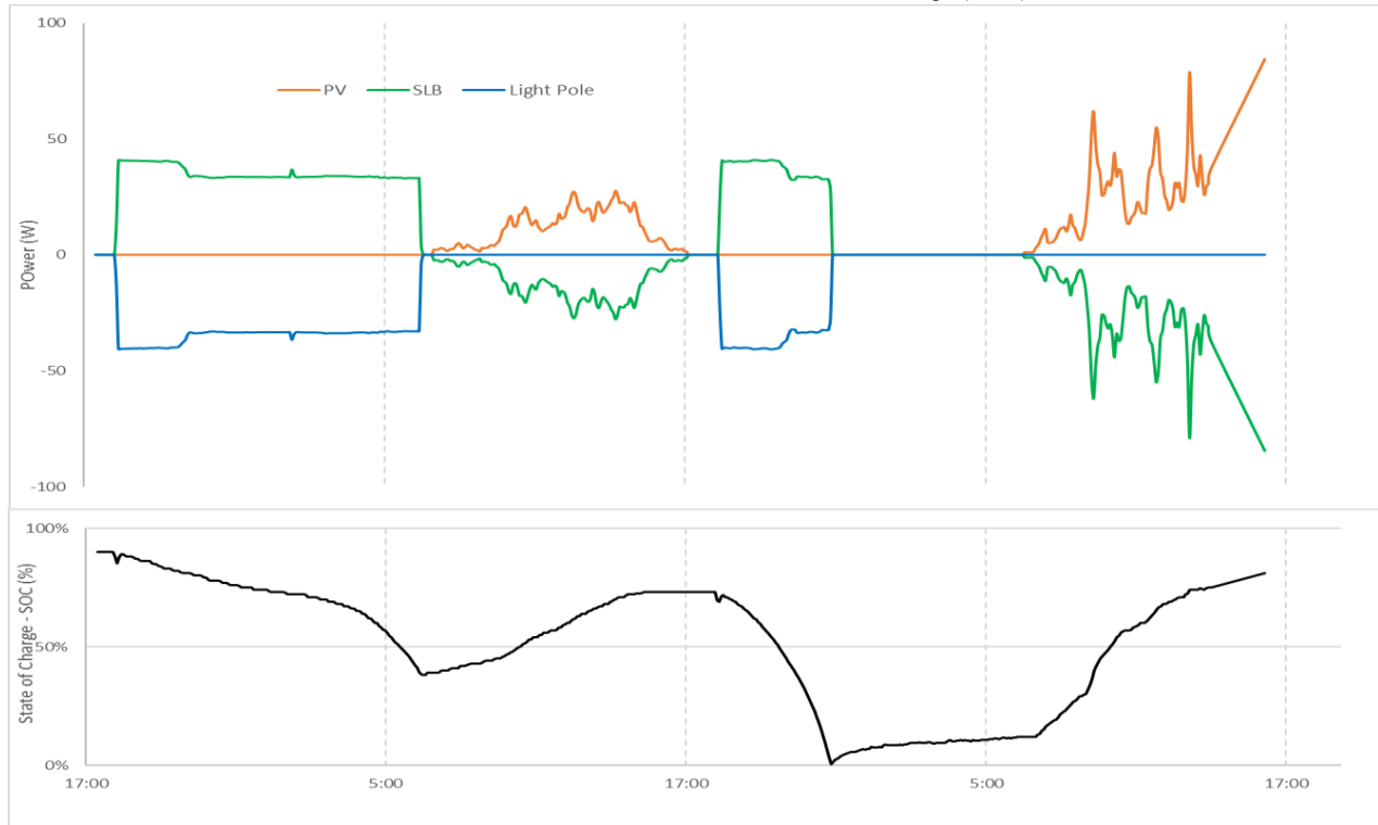
Figure 4. Real-time monitoring of the solar streetlight system during cloudy days, showing the effect of reduced solar generation on the battery's depth of discharge.
