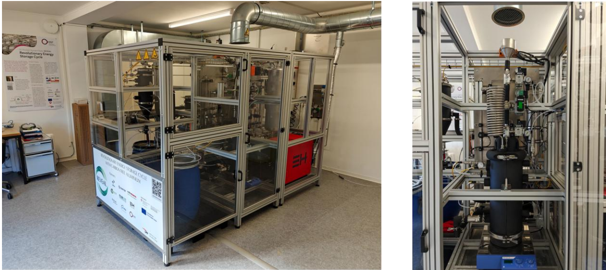
Fig. 3: Pictures of the Alu-to-Energy prototype; Left: entire prototype including all vessels and appliances. Right: reaction vessel, feeding system and condenser.
