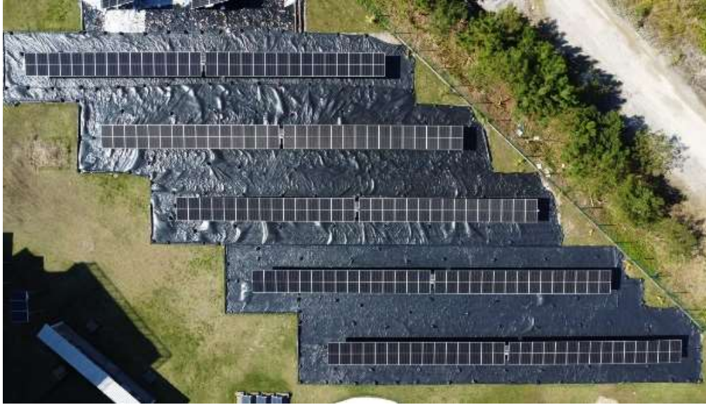
Figure 7: Aerial image of the PV pilot plant used for evaluation of bifacial systems during the baseline period with low-albedo black tarp coverage.
