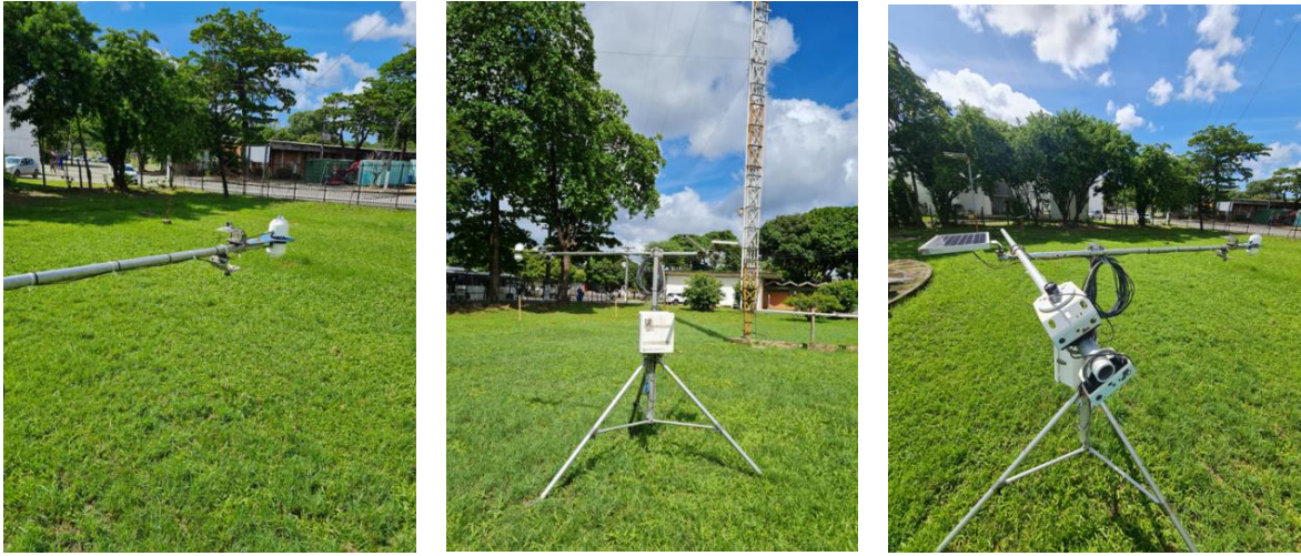
Fig. 1: Weather station with horizontal albedometer and tilted sensors at 30°.
