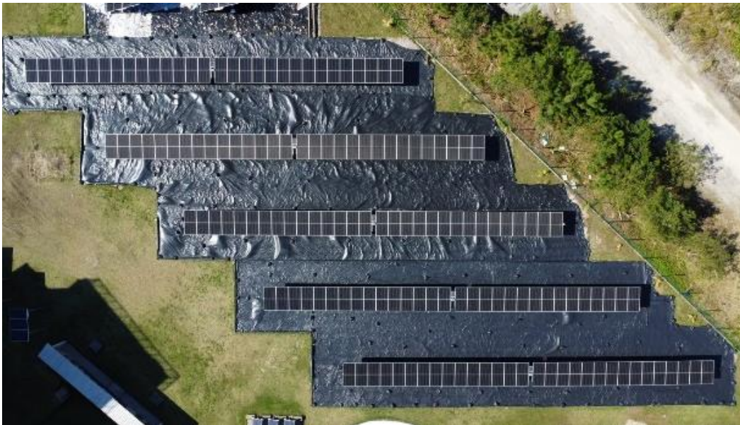
Fig 1: Image of the pilot plant used for the energy evaluation of the reflective ground covers during the baseline period.
