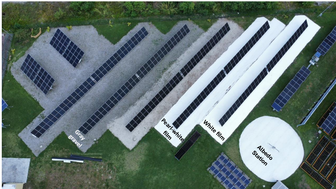
Fig 2: Image of the pilot plant used for the energy evaluation of the reflective ground covers during the normal operation period.
