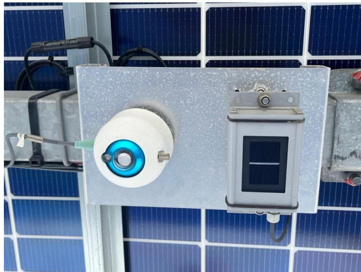
Fig 3: Sensors used for measuring plane-of-array rear irradiance: Class A EKO MS-80S pyranometer (left) and Class A IMT Si-mV-85-PT100 reference cell (right).
