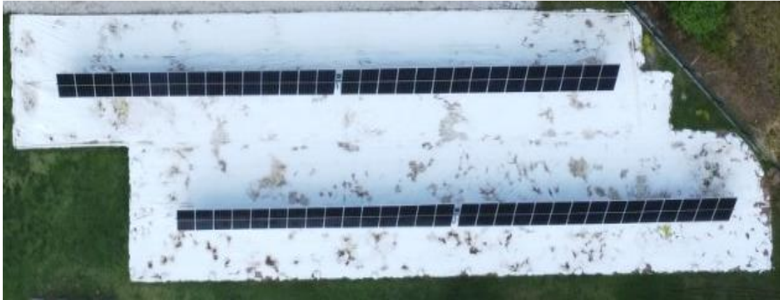
Fig 7: Accumulation of soiling on the reflective films right before the ad hoc cleaning event, used to quantify the associated energy losses presented in Tab. 1.
