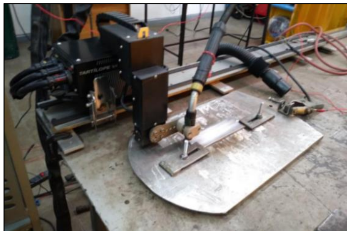
Figure 2: Welding CNC Tartilope V4 that applies the mechanical oscillation in the GMAW process
