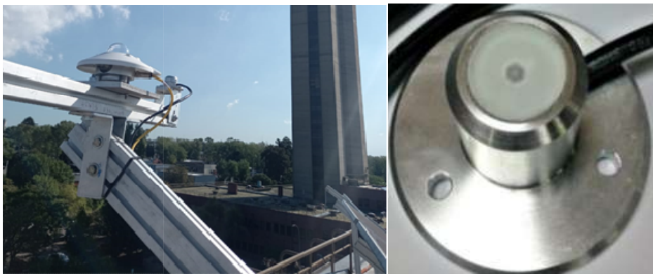
Figure 2: Left, DES UV radiometer and commercial Kipp & Zonen UV radiometer. Right, global radiation (G) radiometer.
