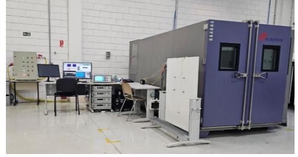
Figure 2: Experimental setup used during the thermal derating tests.
