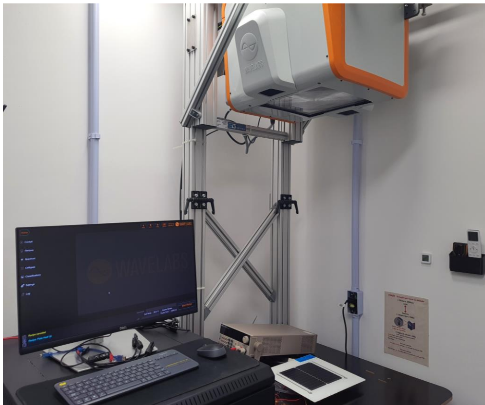
Figure 2: Indoor setup and solar simulator used for controlled irradiance tests at the Fotovoltaica/UFSC Research Laboratory in Florianópolis, Brazil (27.4°S, 48.4°W).
