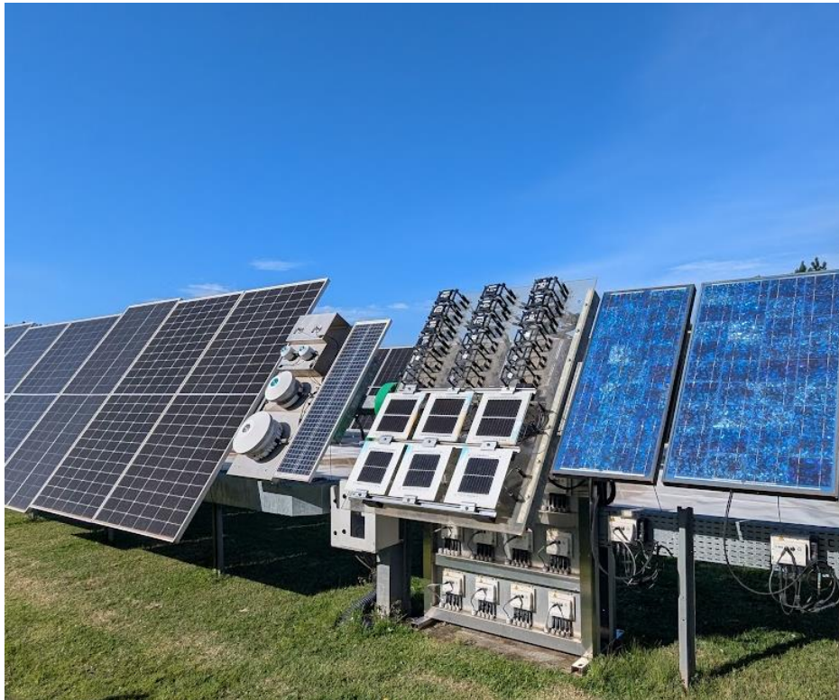
Figure 1: Outdoor measurement setup on a single-axis tracker at the Fotovoltaica/UFSC Research Laboratory in Florianópolis, Brazil (27.4°S, 48.4°W), showing the silicon PV minimodules and sensors used in this study.
