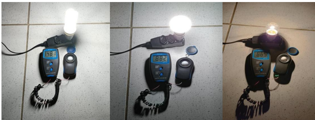
Figure 8: Students conducting measurements of electrical and luminous data to compare lighting efficiency as part of their research project presented at the 2025 MOSCLING Scientific Fair
