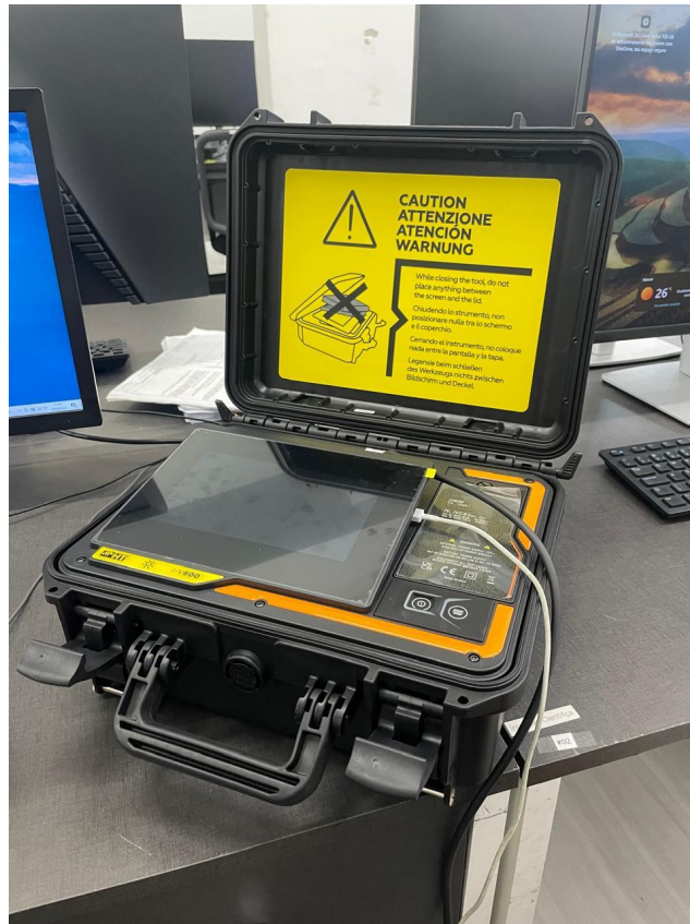
Figure 2: HT-IV600 equipment used for tracing the I-V curves of the photovoltaic modules.
