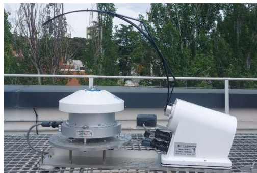
Figure 1: EKO MS-711 RSB spectroradiometer installed at Ciemat (Madrid).
