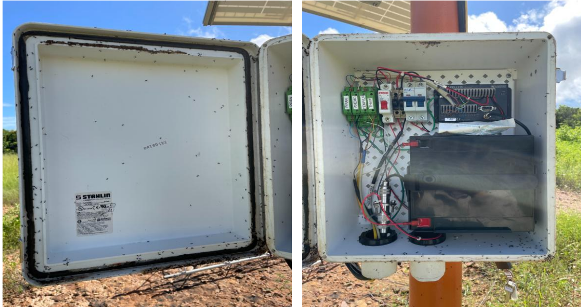
Figure 1: Ant infestation inside the datalogger at the Pau dos Ferros station.
