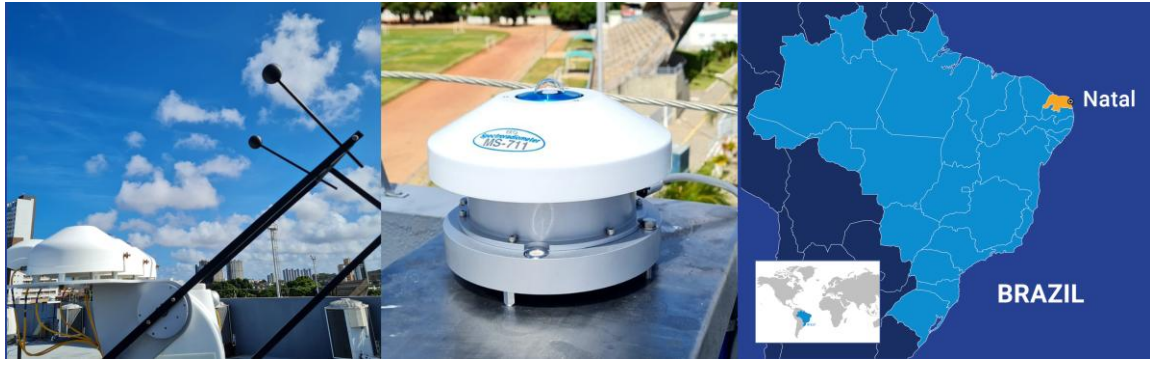
Figure 1: Illustrations of: a) the solarimetric station, b) the MS711 spectroradiometer, and c) a map indicating the study site.
