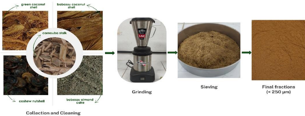
Figure 1: Biomass pretreatment steps: collection, cleaning, grinding, and sieving (Author, 2025).
