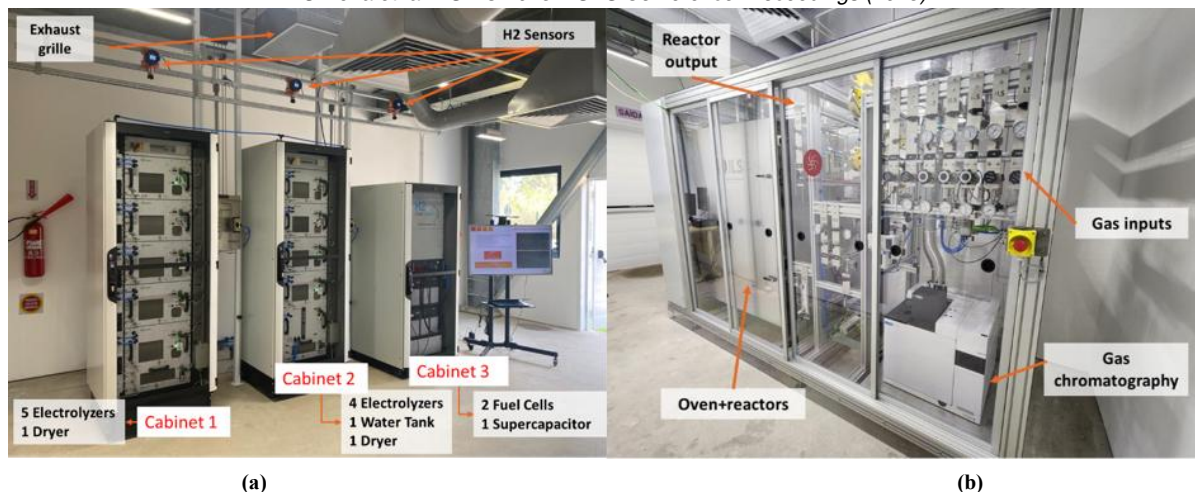
Figure 21: AEM electrolyzers (a) and Haber-Bosch ammonia synthesis reactor (b) at the Green Hydrogen Laboratory at the Fotovoltaica/UFSC in Florianópolis, south of Brazil.
