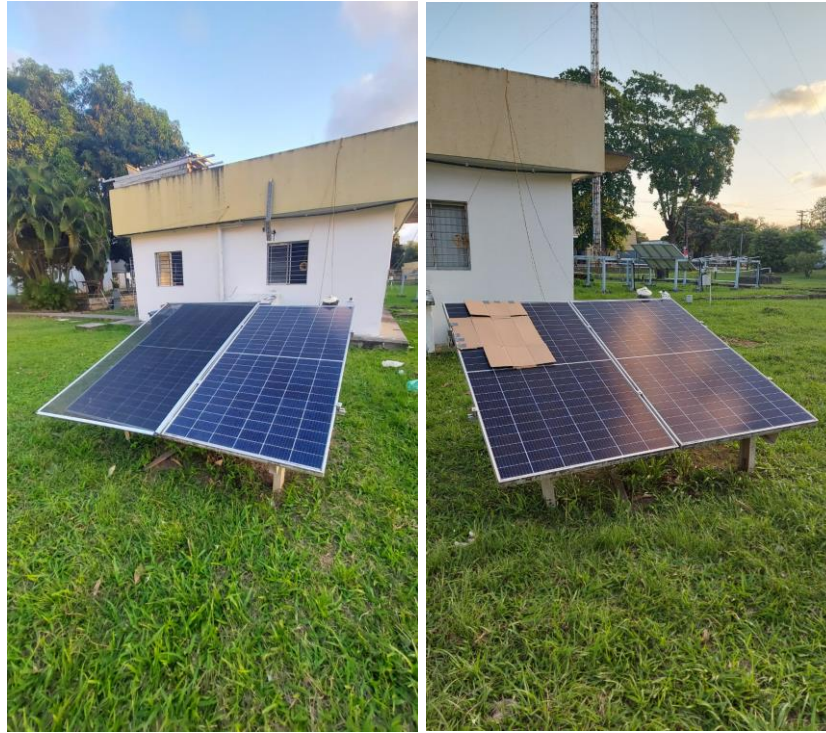
Figure 3: Photographic record of the controlled shading experiments conducted on the PV system. (a) October 10, 2025. A 50% mesh was placed over one PV module for an entire day to simulate partial shading conditions and validate the anomaly detection framework. (b) October 16, 2025. A cardboard sheet was applied to the upper section of another PV module to reproduce a localized shading condition.
