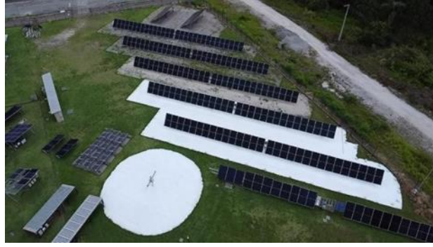
Figure 1: Aerial view of the PV pilot plant at UFSC, showing bifacial PV trackers installed over gravel (top of the image) and geomembrane surfaces.
