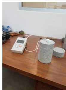
b) Measurement in cellular concrete
