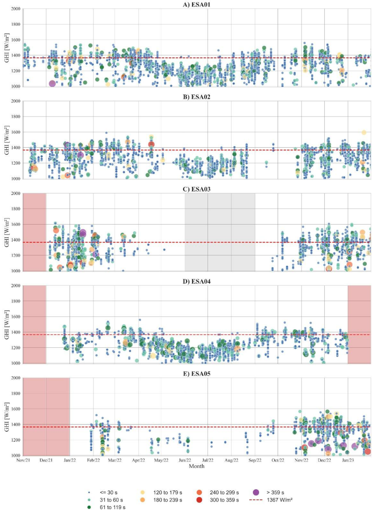
Figure 6: Distribution of the duration of overirradiance events at second resolution at stations (a) ESA01, (b) ESA02, (c) ESA03, (d) ESA04, and (e) ESA05. The gray bar represents the absence of OIE events, while the red bar represents that no data is available.
