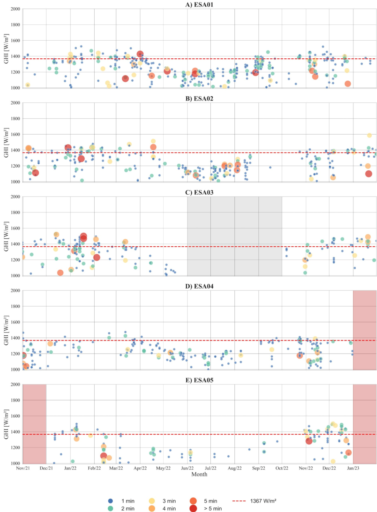
Figure 5: Distribution of the duration of overirradiance events at minute resolution at stations (a) ESA01, (b) ESA02, (c) ESA03, (d) ESA04, and (e) ESA05. The gray bar represents the absence of OIE events, while the red bar represents that no data is available.
