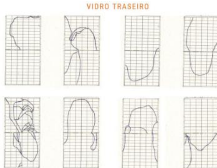
Figure 8: Pattern of cracks found in bifacial modules (Adapted from Azevedo et al., 2024)
