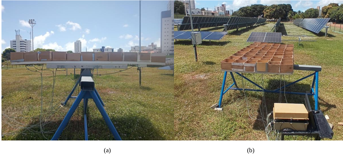
Figure 5: a) Side view of the static load test and (b) Illustration of the photovoltaic module under the effect of the distributed load
