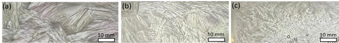
Figure 9: Crystal grain size of 0.1 wt% ZnO-doped CCH for samples cooled at (a) 25 degrees (b) 8 degrees and (c) -5 degrees.
