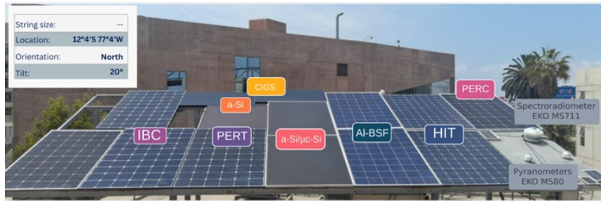
Fig. 1: Performance and reliability system at the Outdoor Photovoltaic Research Laboratory.
