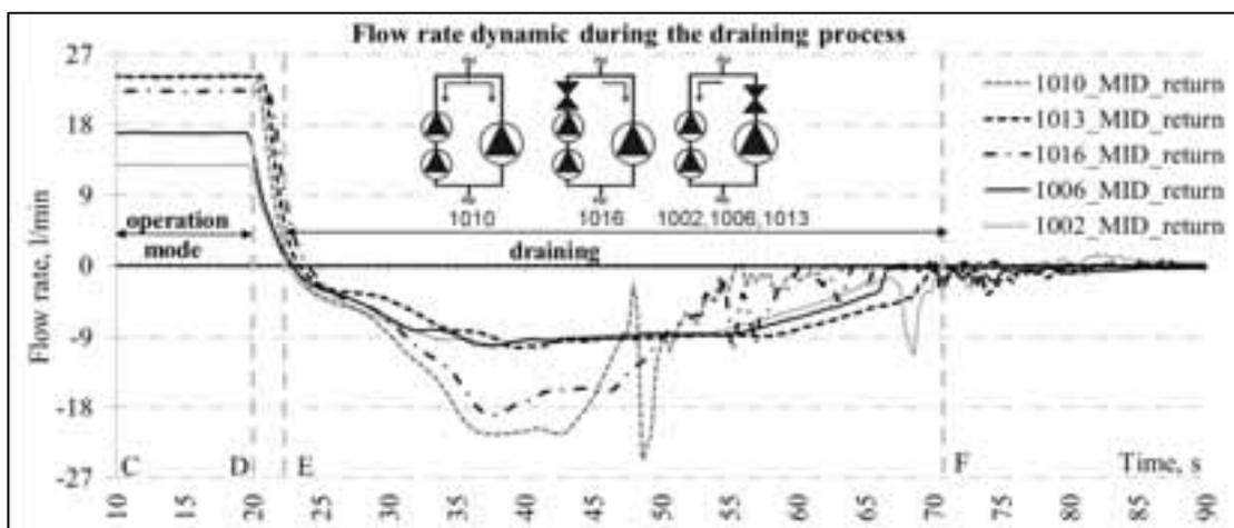
**Fig. 9: Flow rate dynamic during the draining process**
