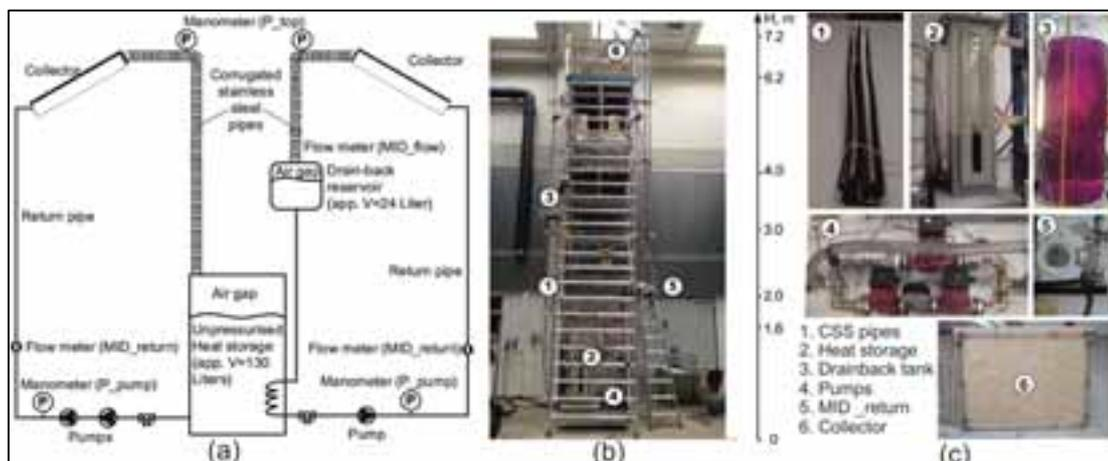
**Fig. 3: Hydraulic scheme (a) of the experimental setup (b) and hydraulic components (c)**
